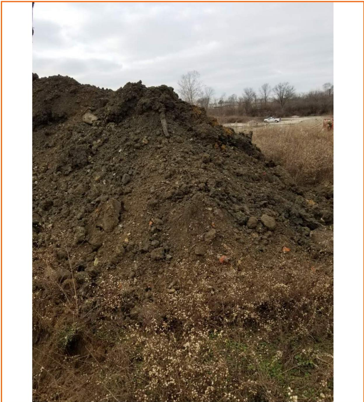
Photo 9 - Excavated fill at Test Pit TP-10
